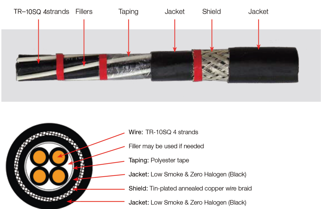
YHSPD Cable (TR Series) Cross-sectional view and composition
